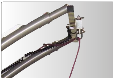
Fall stop at the crossbar of the safety arch
